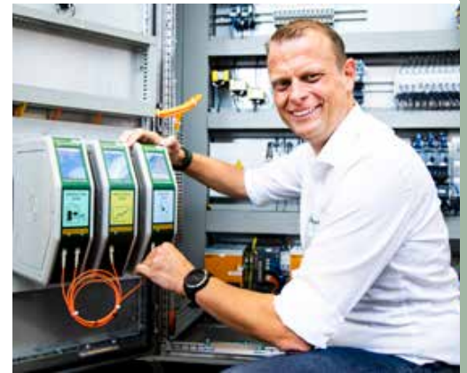
Secure communication: Gert Hansen demonstrates the modules of the Pharma Platform. Its extra-secure zone can send data out but cannot receive any data.
